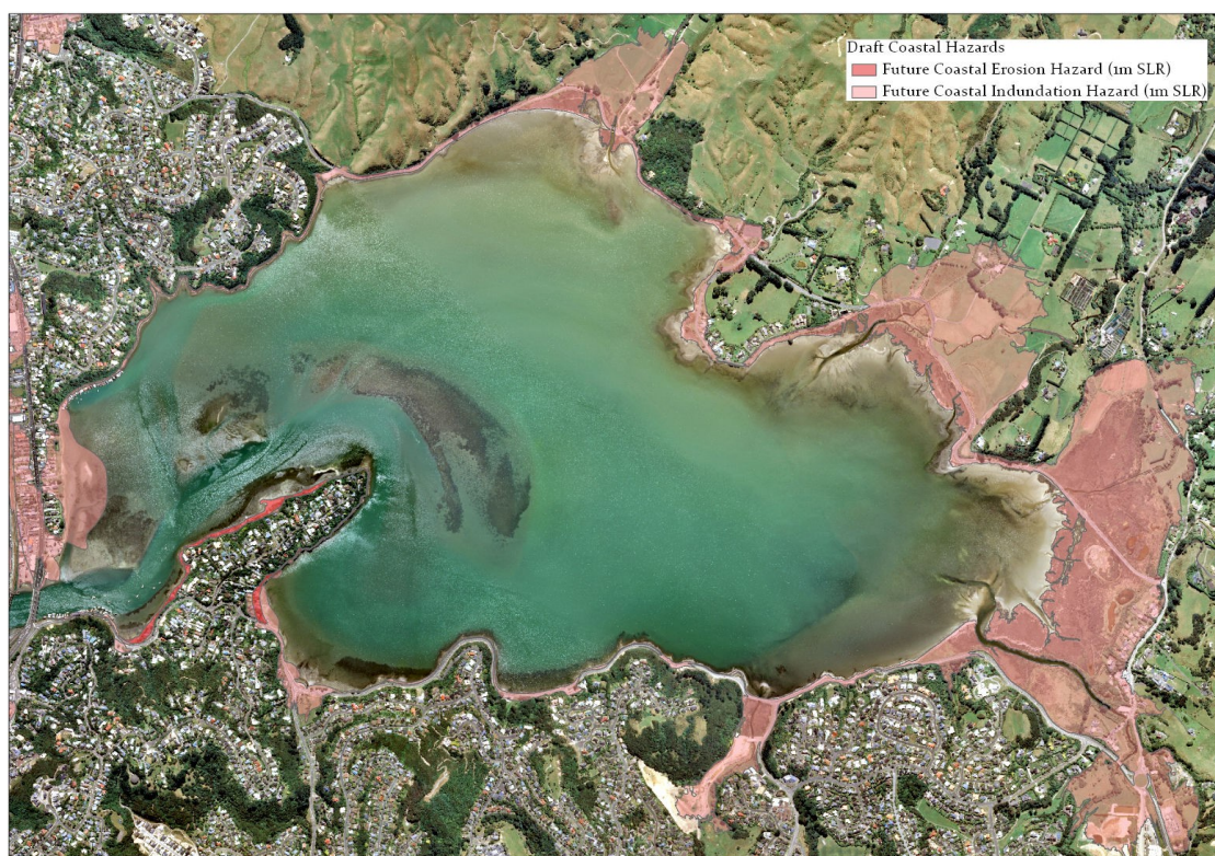
This image shows the future coastal erosion hazard (dark pink) and future coastal inundation hazard (light pink). Photo courtesy of Porirua City Council
